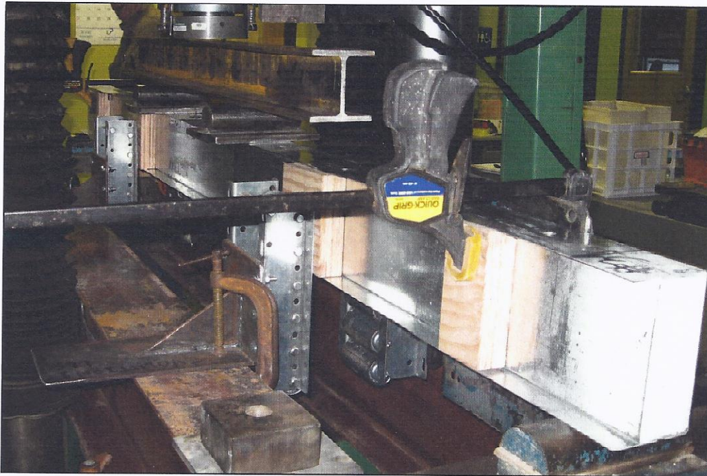
Figure 6 - Strong Axis Bending Test before Loading
