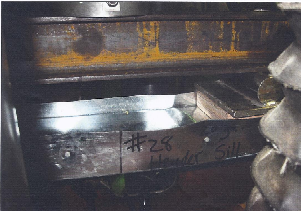
Figure 5 – Weak Axis Bending, Web at Failure
