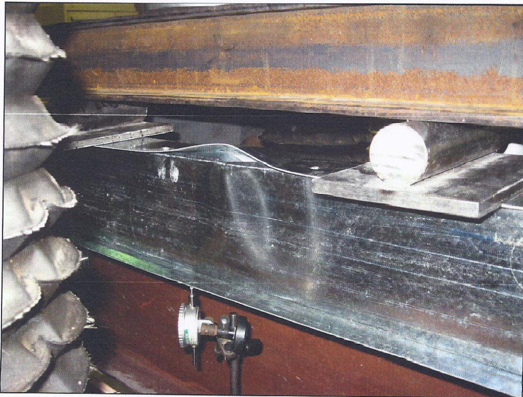
Figure 7 - Strong Axis Bending, Flange at Failure
