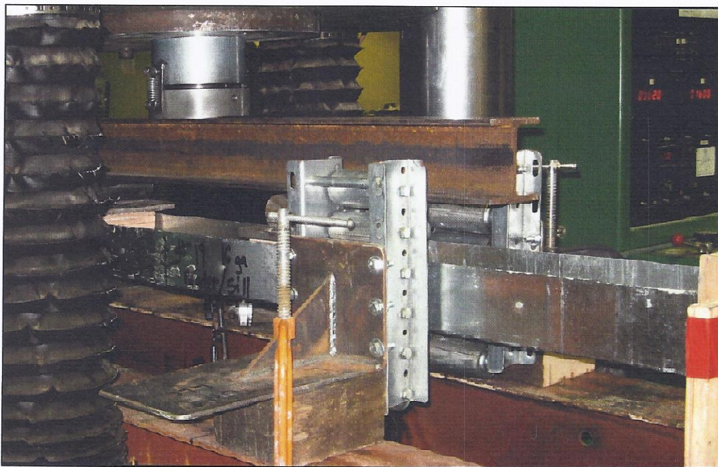
Figure 3 – Weak Axis Bending Test before Loading
