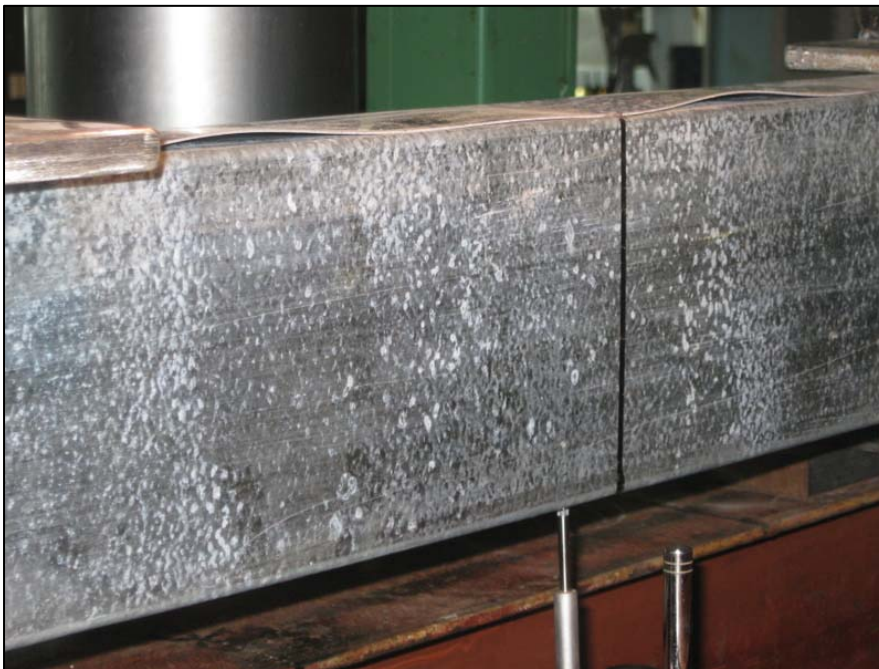
Figure 3 – Outer Flange Buckling
