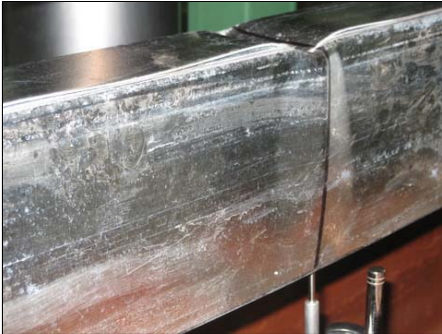
Figure 4 – Flange at Failure at Mid-Span
