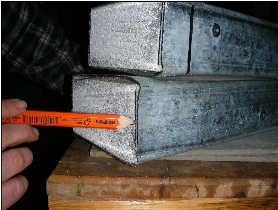
Figure 5 – Flange at Failure
