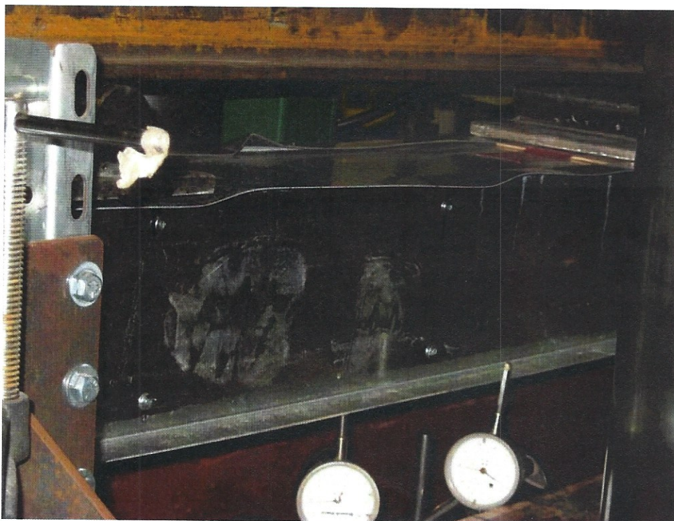
Figure 7: Weak Axis Bending: Compression Flange Buckling of Capping Tracks
