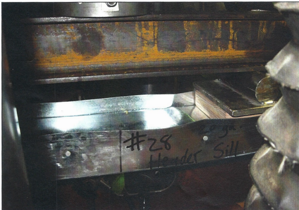
Figure 5 - Weak Axis Bending, Web at Failure
