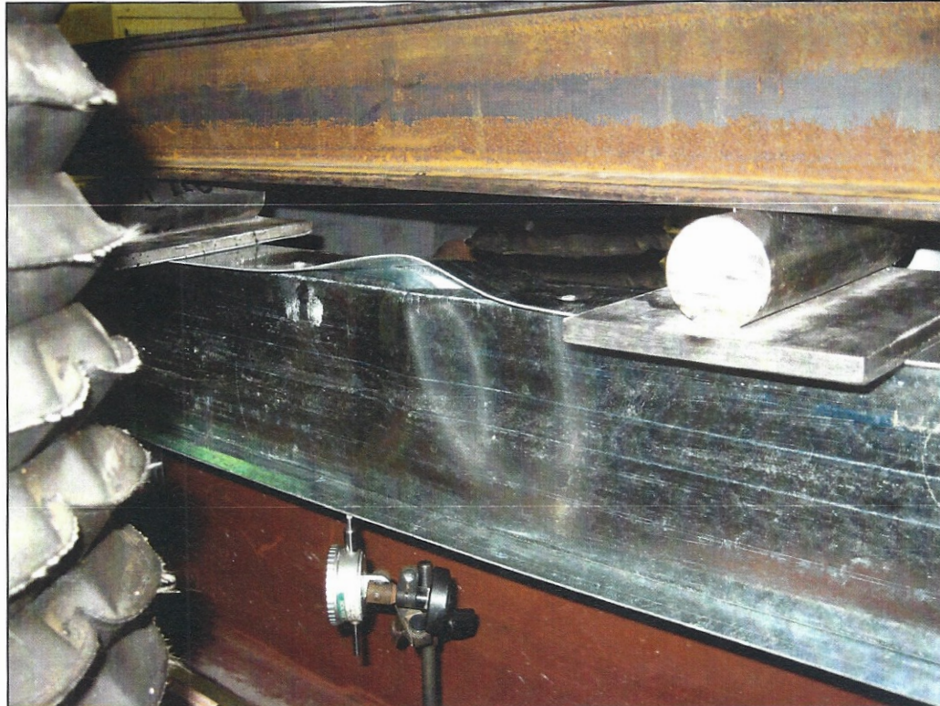
Figure 7 – Strong Axis Bending, Flange at Failure
