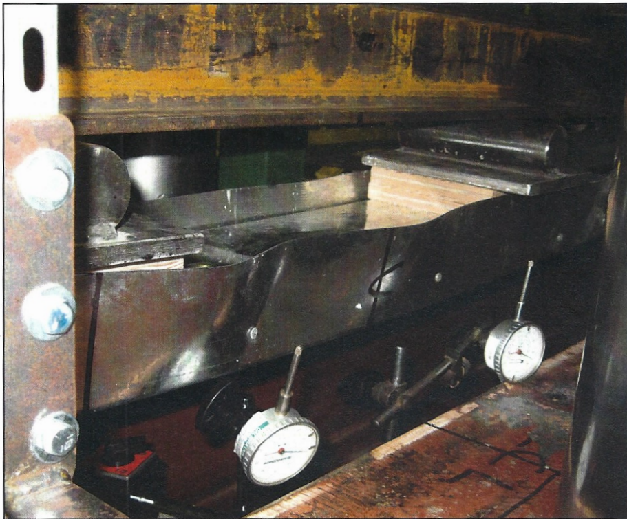
Figure 4 - Weak Axis Bending, Outer Flange Buckling
