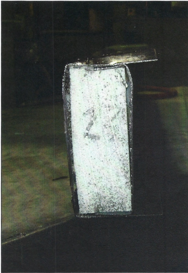
Figure 8 – Strong Axis Bending, Web Distortion at Failure Plane
